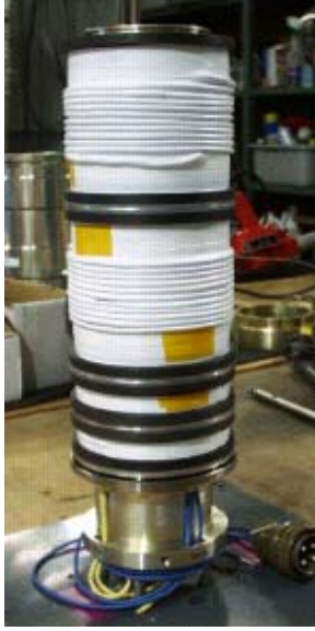
Figure 7. Transformer Inner Core
